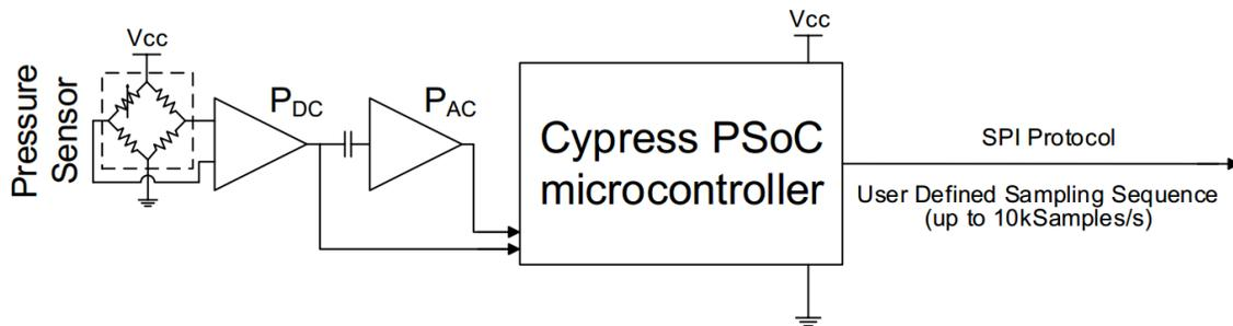
Figure 2 - Electrical schematic of the NumaTac
